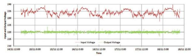
The above is an actual log of input voltage (widely fluctuating red graph) and controlled output voltage (green graph) in a large fabrication workshop fed by our Voltage Power Optimiser.
